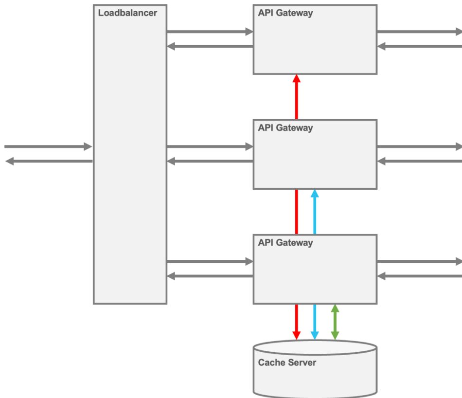
Image: Gateways sharing a cache server like Redis to manage a unified state
